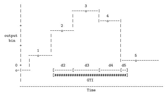
**Interpolated model:** Aspect records denoted by **o** are in the same coordinates as before, GTI is the same. Now points are to be connected by linear segments. The +-marks roughly indicate when the segment crosses an output bin (or is midway between records if in the same bin), and align with duration boundaries.
